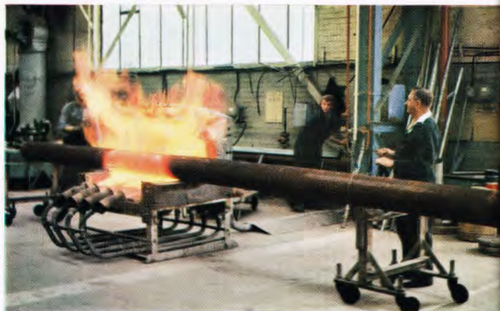
A pipe being heated prior to hot bending in the Plumbers' Shop
